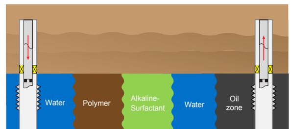
Figure 1 - Alkali is injected to react with the organic acid in the oil to produce in-situ surfactant to reduce  $S_{orw}$ . Synthetic surfactant and Polymer flood are also injected to further reduce  $S_{orw}$  and improve mobility control.
